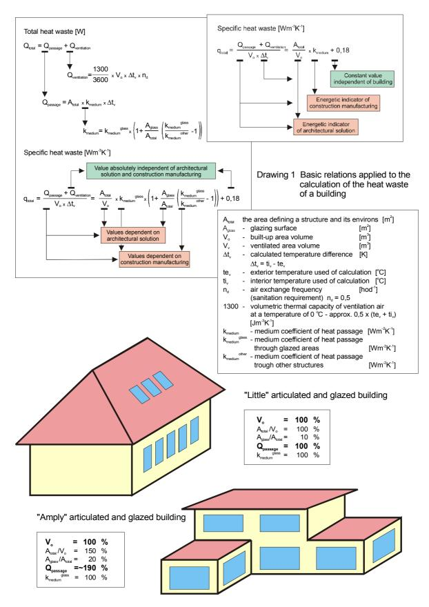
Drawing 2 The effects of an architectural solution and construction manufacturing on thermal passage waste
